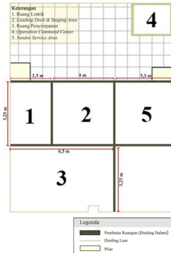
Figure 6. PDII-LIPI's data center space and support space proposal looked from top
