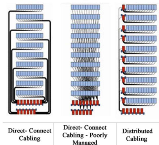
Figure 11. Illustration of wiring method comparison (Cisco System, Inc, n.d.)
