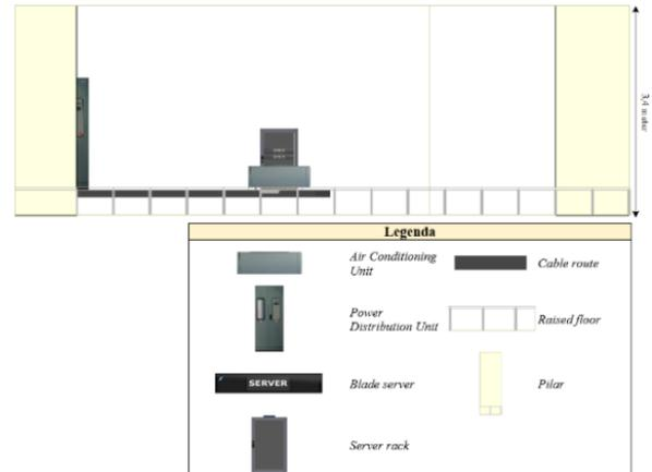
Figure 4. Ceiling high PDII-LIPI's data center proposal
