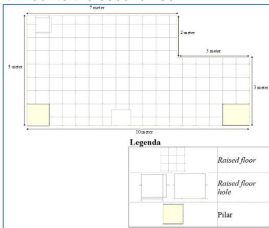
Figure 3. New PDII-LIPI's data center space proposal looked from top
