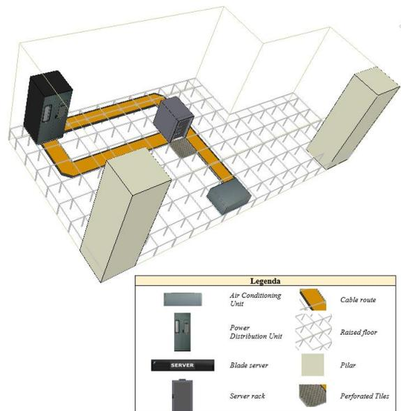
Figure 7. Three-dimensional shape of the data center space along with the proposed plan of the data center room with tools
