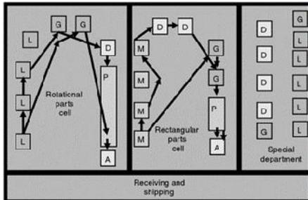
Figure 4 A GT-Base Of Cellular Manufacturing Layout
