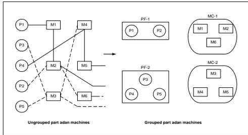
Figure 6 The Physical Machine Layout
