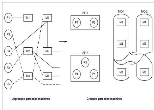
Figure 7 The Logical Machine Layout
