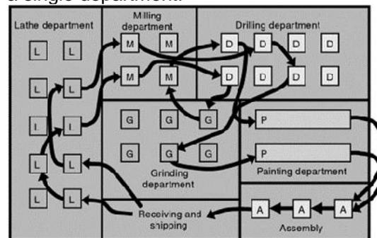
Figure 3 The Layout Process
