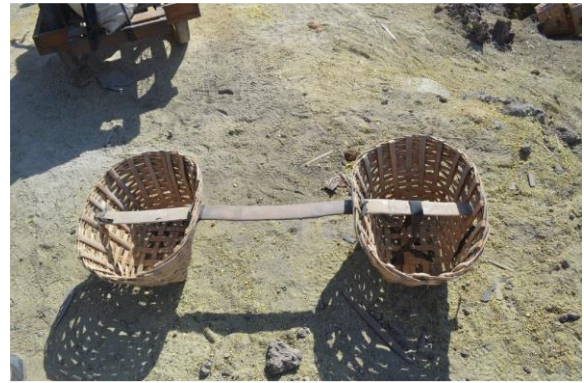
Figure 1 Sulfur basket as existing sulfur conveyance
