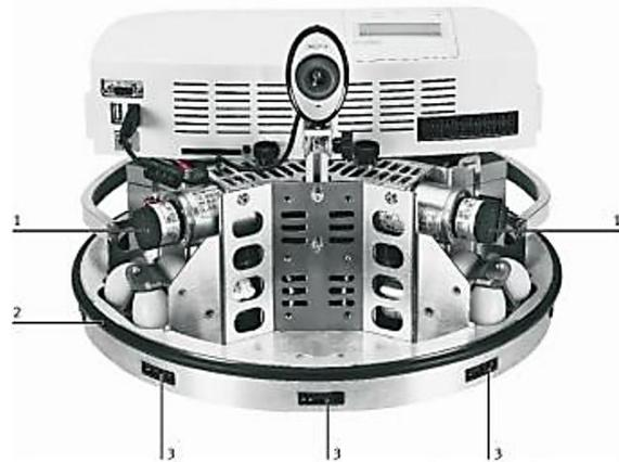
Figure 2. Three unit sensors of Robotino®: (1) incremental encoder, (2) anti-collision sensor, and (3) distance measuring sensor
