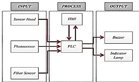
Figure 7. Design of control system machine
