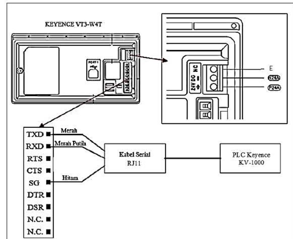
Figure 9. Wiring diagram of Keyence VT3-W4T
