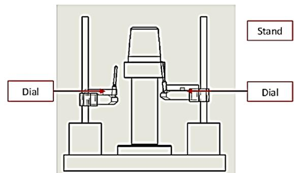
Figure 3. Inspection jig before improvement
