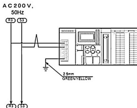
Figure 8. Wiring of PLC diagram power
