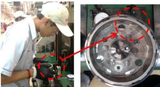
Figure 5. the process of boss rotor check
