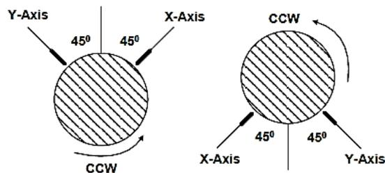
Figure 2 Measurement with proximity probes on shaft
