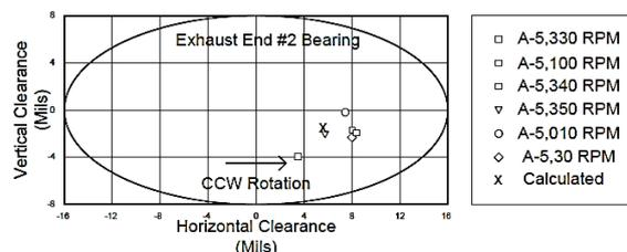
Figure 6 Corrected Proximity Probe Gap Voltages At Turbine Exhaust End #2 Bearing
