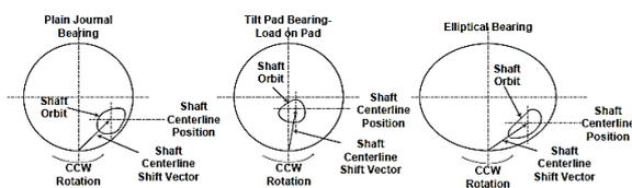
Figure 3 Shaft centerline position on journal bearings at inlet end #1
