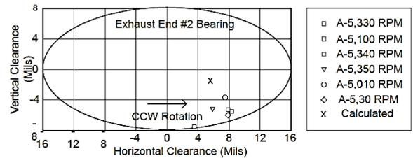
Figure 4 Shaft centerline position on journal bearings at exhaust end #2
