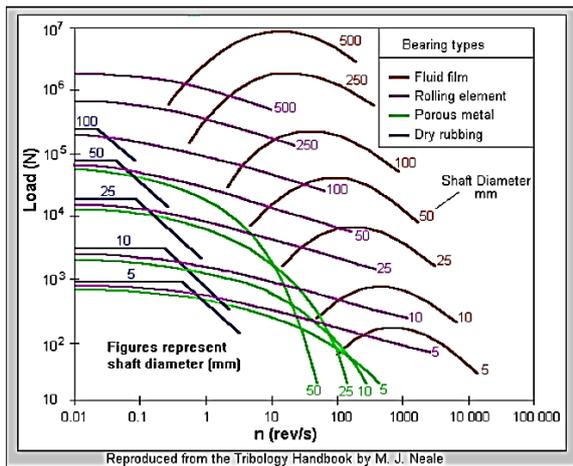
Figure 1 Operating ranges for different types of bearing
