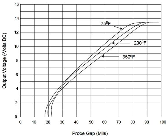
Figure 5 Variation in calibration curves at temperatures of 75, 200, and 3500F
