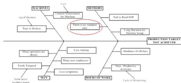
Image 7 Cause and Effect Diagram Resulting from Unmet Production Target
