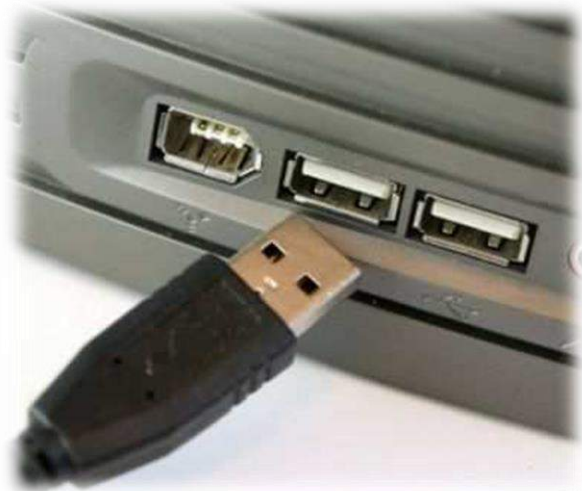
Figure 1. USB port on Computer is a Example of Poka Yoke (e)
