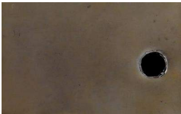
Figure 11. Plating result with stirring (PGC solution without claryx)
