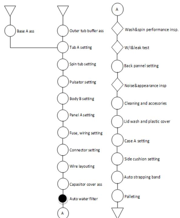
Figure 1. Process chart of washing machine assembly
