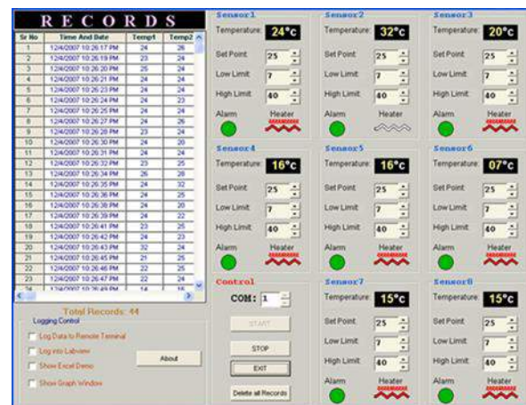
Figure 9. Reporting Result Data on EMS-SCADA
