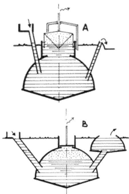
Figure 1: Types of bio-digester (A) floating drum (B) fixed dome (Energypedia, 2012)
