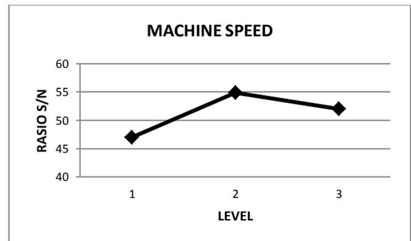
Figure 4. Machine Speed *Main Effect Plot* for S/N Rasio
