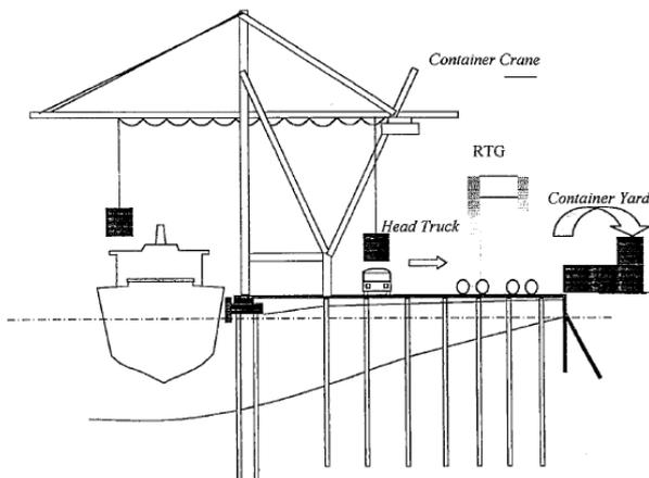
Figure 2 Illustration of loading and unloading at the Ocean Going container port (009)
