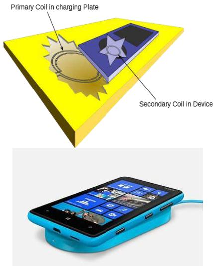
Figure 3. Wireless charging Workflow
