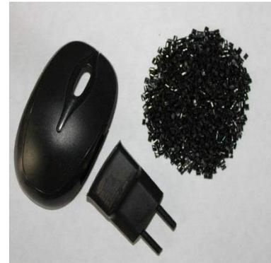
Figure 4. Polycarbonate/Acrylonitrile Butadiene Styrene (PC/ABS) plastic
