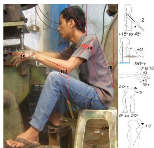
Figure 6. Work Posture in conducting the Blanking process
