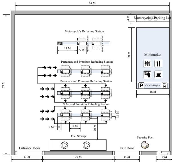
Figure 4. The layout of queue line for Scheme 2
