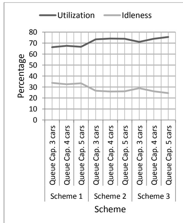
Figure 6. The average of Utilization and idleness rate for each scheme with different queue capacities.
